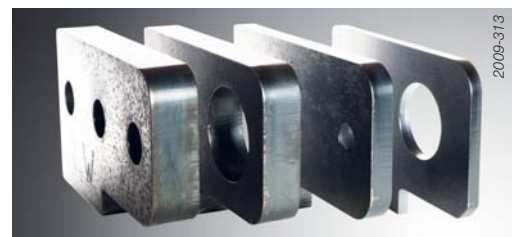
HP cuts - carbon steel O 2 /Air
