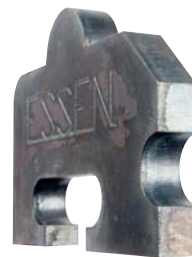
Carbon steel - 25 mm oxyfuel process
