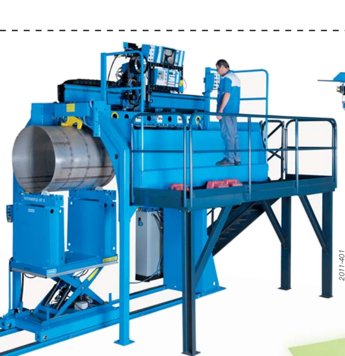
The Seamer benches for longitudinal weld of plates or vessels.
