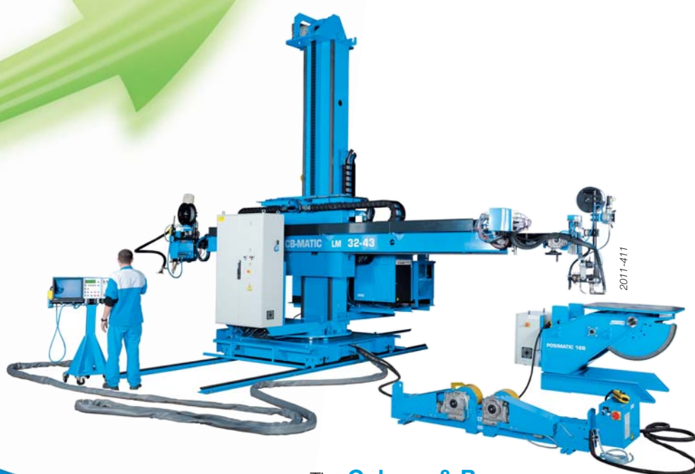
The Column & Booms to weld large tanks with any processes.
