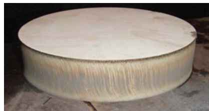
Stainless steel - water vortex - 60 mm
