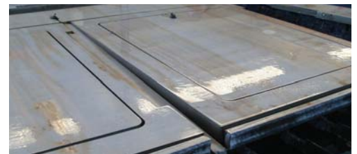
Stainless steel - water vortex - 60 mm
