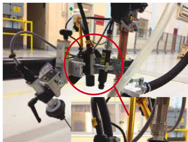
Camera installed onto bracket for welding torch
