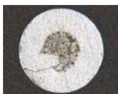
Elgacore Matrix wire seam cross section ultra-consistent seam, smooth and tight.
