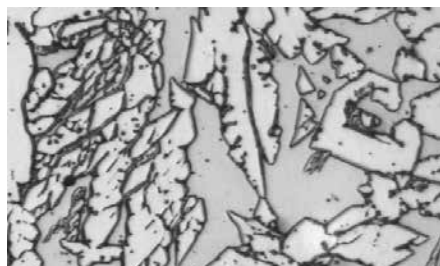
Duplex Weld Metal, 200x
