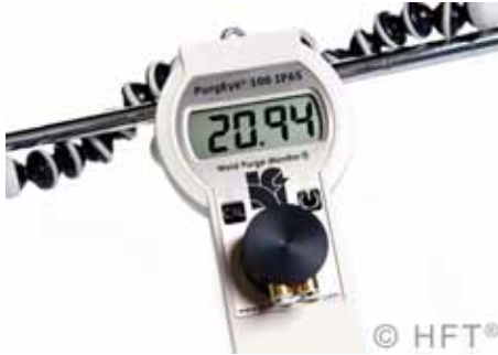
PurgEye® 100 IP65 to indicate from 20.94% to 0.01% (100 ppm).
