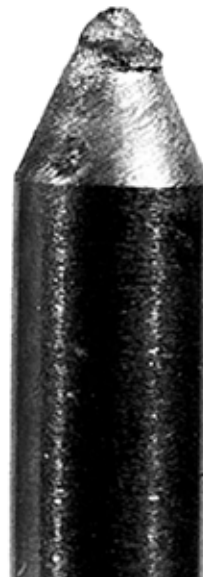
2% Thoriated Tungsten after 20 automatic welds
