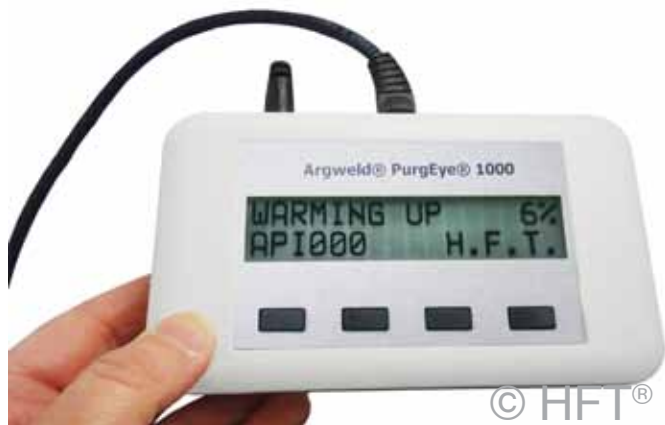
Portable 'handy' Weld Purge Monitor® to read from 1000 ppm down to 10 ppm
