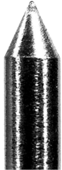
MultiStrike® Tungsten after 200+ welds
