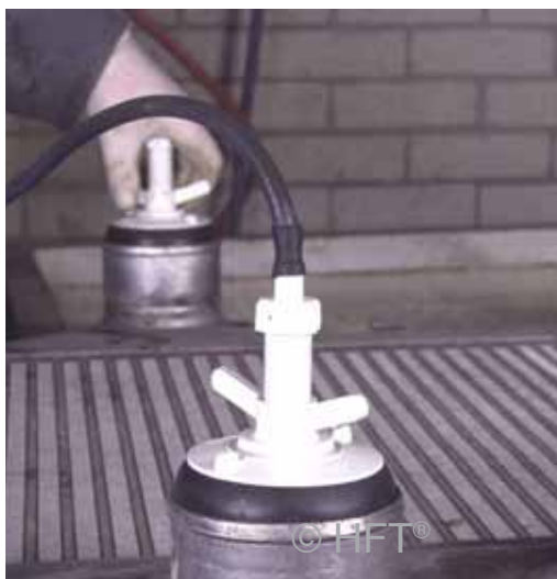
Hollow shaft plugs being prepared for testing an intercooler
