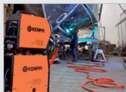
Traditional motor pistols and spool gun designs increase weight and strain on the operator's wrist and are limited by their distance, filler wire, or volume welding capability. The SuperSnake GT02S resolves all of these issues, while reducing the weight and strain on the operator's wrist by using standard welding guns.
