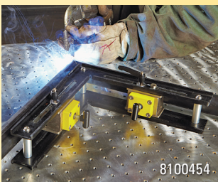
Magnets positioned away from joint to prevent arc blow.
