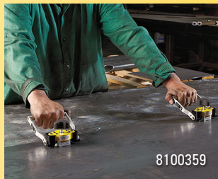
Pivot handle allows use as a hand lifter or a sheet dragger.
