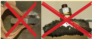
Stays clean. Turn off Magswitch and wipe away debris.
