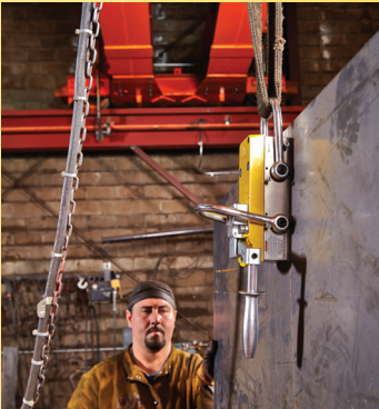
Use the single hook to lift in shear.
