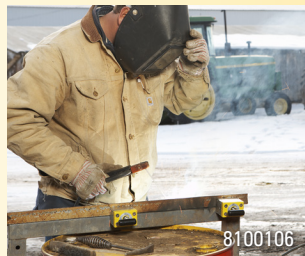
Align two pieces of steel – flat or round.
