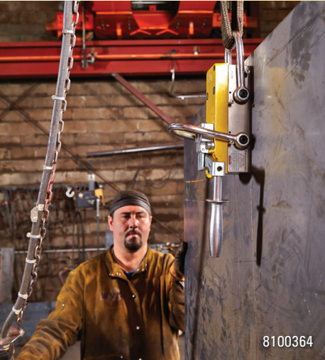
Use the single hook to lift horizontal to vertical.
